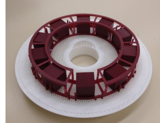
Figure 31: 3D printed sub-scale mockup of the SOEPSS
