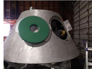
Figure 4. Initial Condition of the Almaz EEUM with damaged hatch
