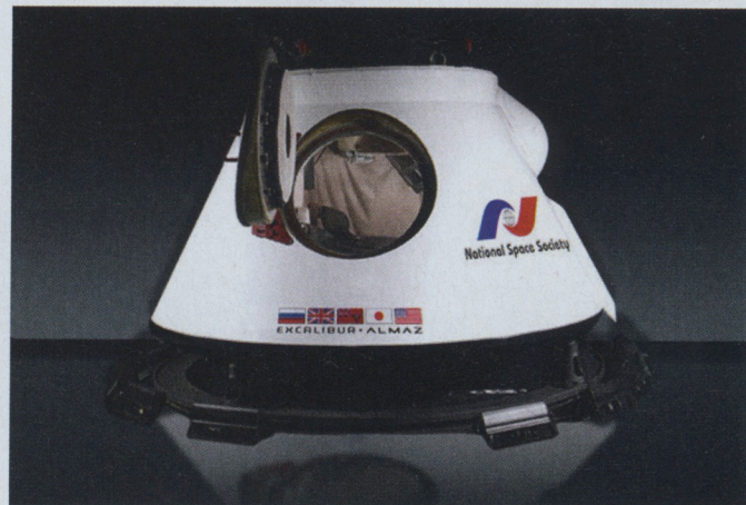
The Almaz crew capsule looks much like an Apollo capsule, but has a slightly smaller habitable volume for its crew of three.
